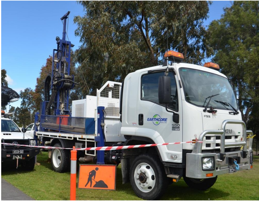
Example of a truck with a drilling rig used to undertake bore holing
