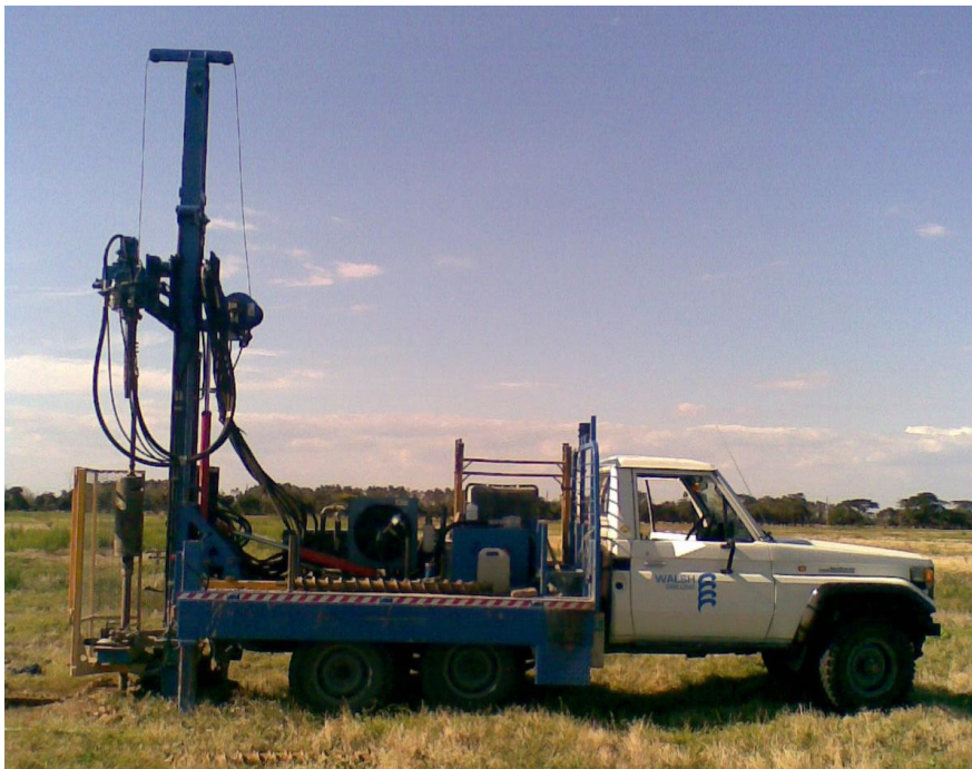
Example of a 4WD with a drilling rig used to undertake bore holing
